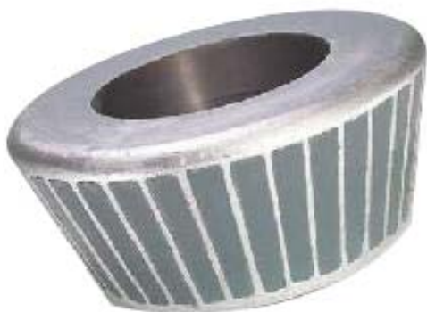
Picture of vertical mill parts- rollers and table liners
