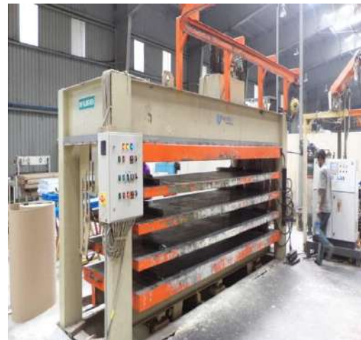
Putting into Hot Press (4 day light pressing)
